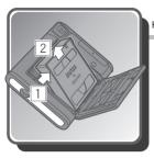
How to remove the INSTAX SQUARE instant film cartridge once all film sheets have been used.
